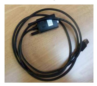
You have to connect the RS232-USB cable converter in the RS232 serial port on the Sirius (see picture below).
