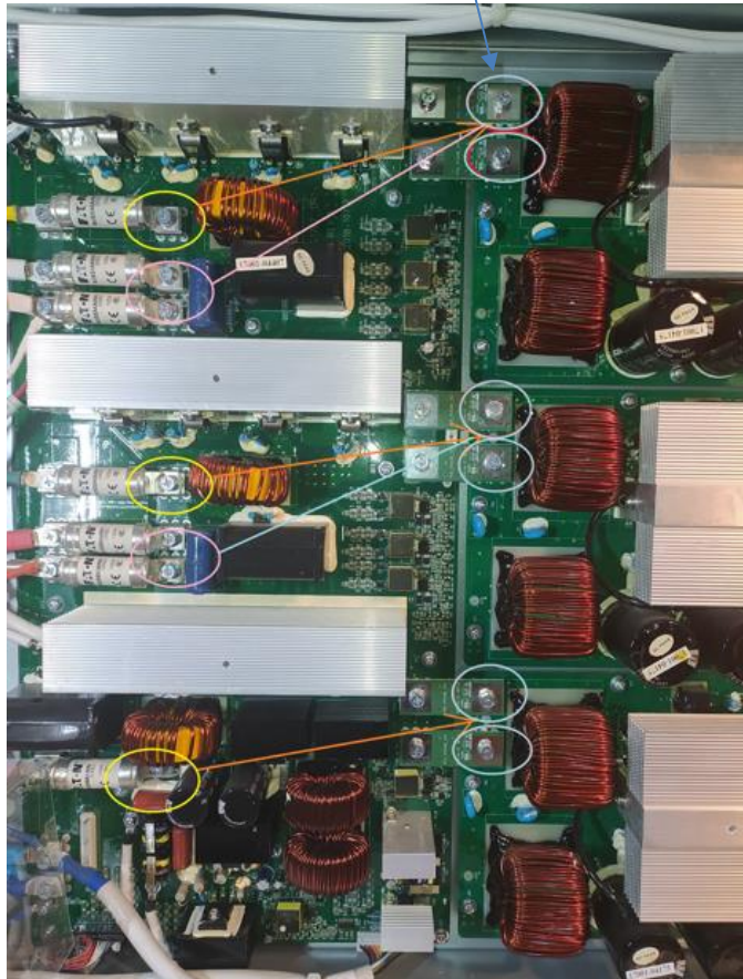
Main input SCR detection Tab.3-3-2-
