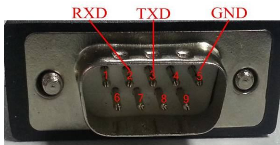
Pic 1-3. Male type pins definition of RS_232 Port
