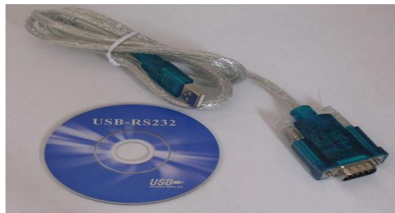
Pic 1-8. USB-RS_232 cable and drive program
