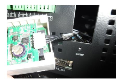
1.3 Insert the SNMP card in the free slot present.
