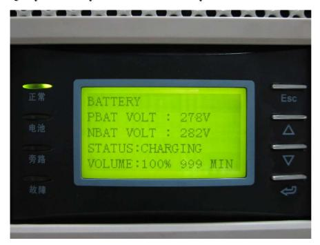
In the Battery information menu, we can find charge status valued =100%, and remaining battery backup time = 999 mintues. The battery remain time for MUST UPS is based on 9Ah battery set and the minimum number is "2" per battery set (total q'ty: 40pcs, 20pcs in string and 2 strings in serial connection per battery set).
