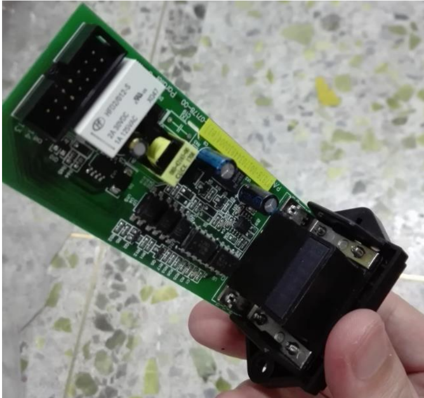
Step 3. Insert parallel board into parallel box
