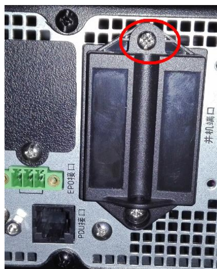
Step1. Unscrew the parallel cover.
