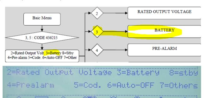
3) To change battery voltage you need to change Battery type from std setting to custom setting, to do it change Battery type from "1"=std to "0" =custom, using key 2 (2 = -1 in this menù)
