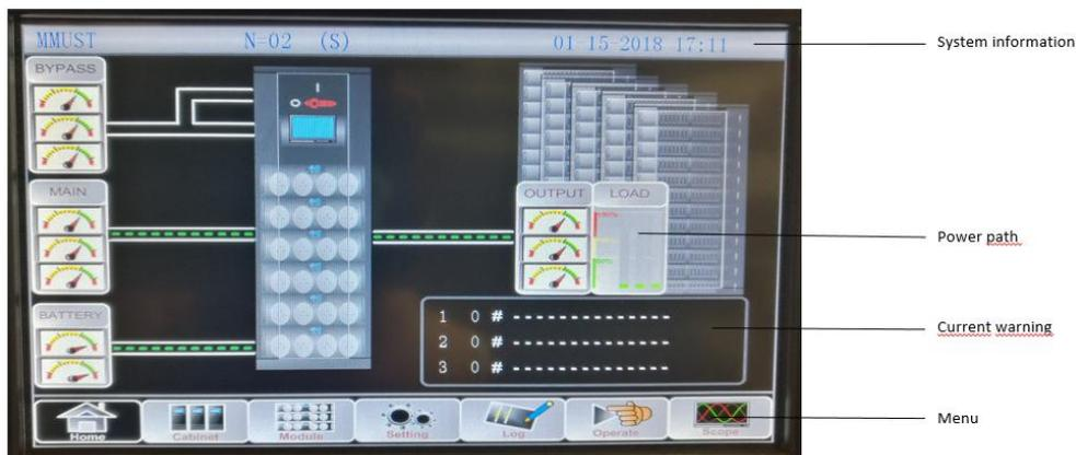
Fig. 7-2: Display LCD principale
