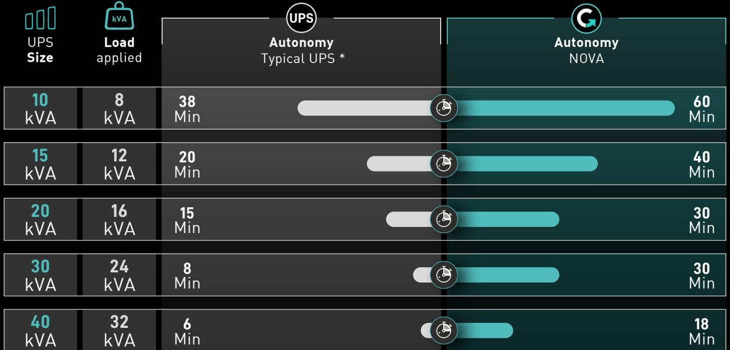
\* Threephase UPS with 2 internal strings of 40 batteries (12V / 9 Ah)
