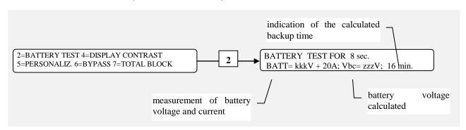
This activates the cycle to check the state of efficiency of the battery, which lasts 8 seconds. Press key 8 to interrupt the test and return to the basic menu before this time has elapsed.
