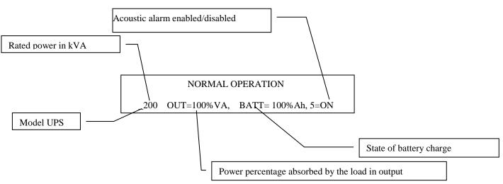
The message OUT changes to BY when the load is not powered from the inverter (normal operation) but from the mains through the by-pass line.
