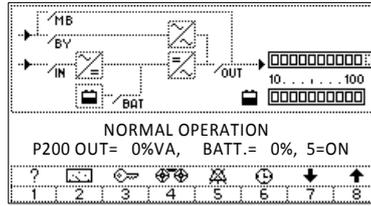
if there are alarms, the active ALARM messages are displayed one at a time for a few seconds.
