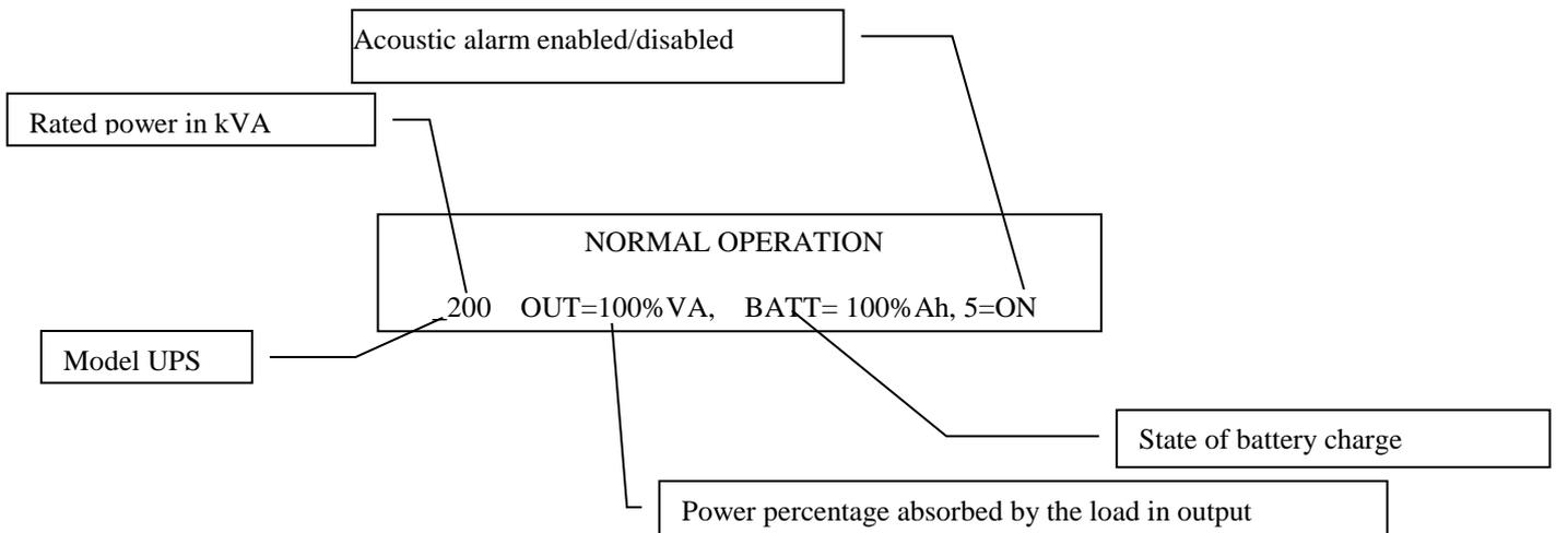
The message OUT changes to BY when the load is not powered from the inverter (normal operation) but from the mains through the by-pass line.
