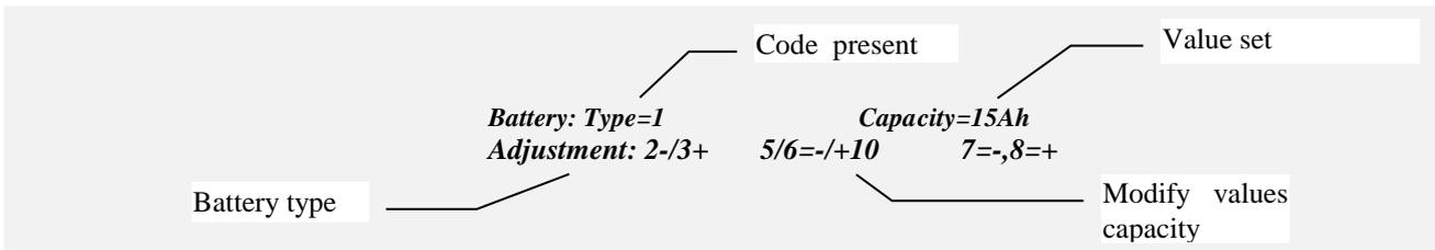
On first installation the rated capacity value of the connected battery must be inserted; this value is usually printed on the battery container.
