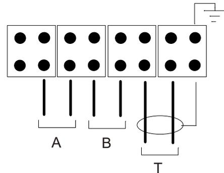
A = connection to external output CPS switch auxiliary;
