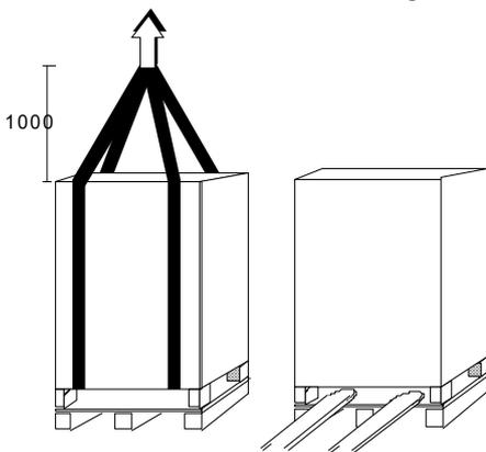
RIMOZIONE DEL PALLET / TO REMOVE THE PALLET
