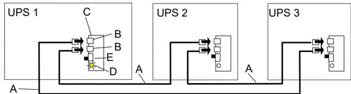
**The connectors must remain connected even if the CPS is switched off**
