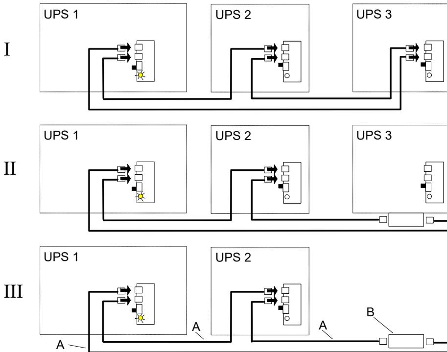
A) CPS parallel cable type RJ45
