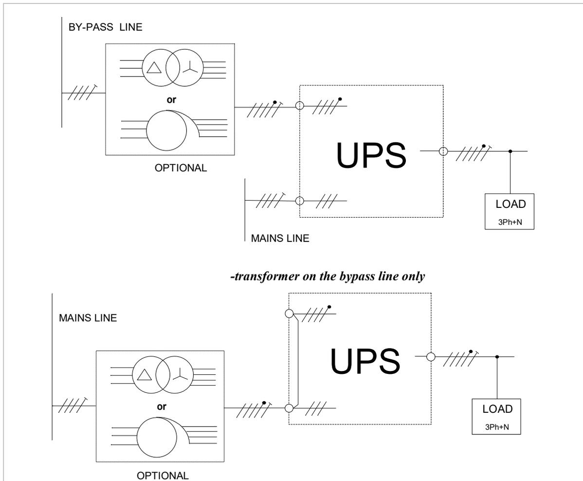
*-The transformer supply bypass and mains lines*
