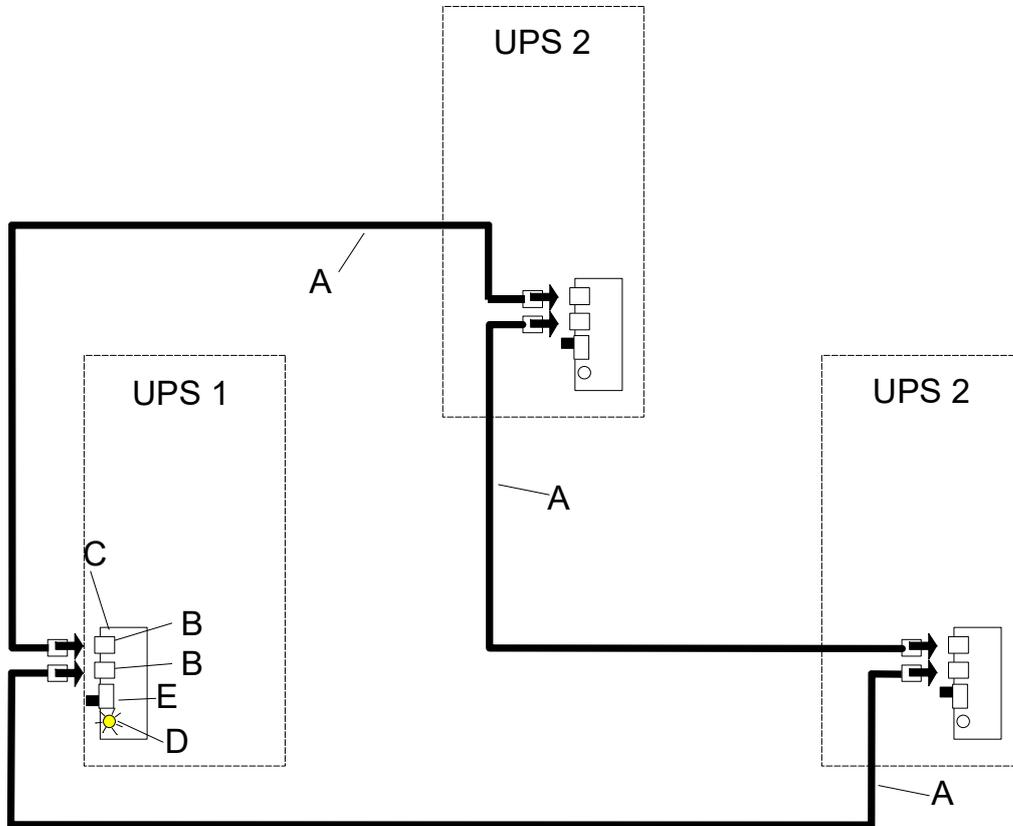
To add other parallel CPSs, a “CPS PARALLEL CABLE” must be added for each new CPS connected.
