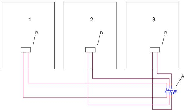
A) EPO switch (refer to the “REMOTE CONTROL & SIGNALS” section earlier in this manual status to determine the relevant connection pins)
