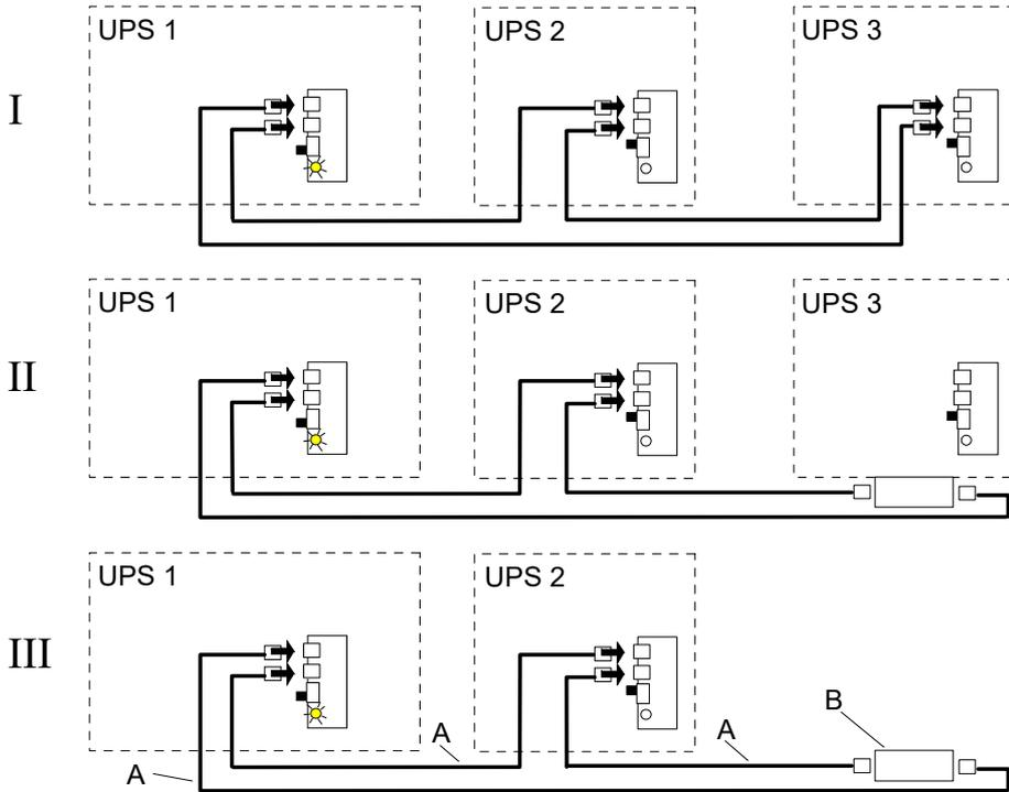
A) CPS parallel cable type RJ45
