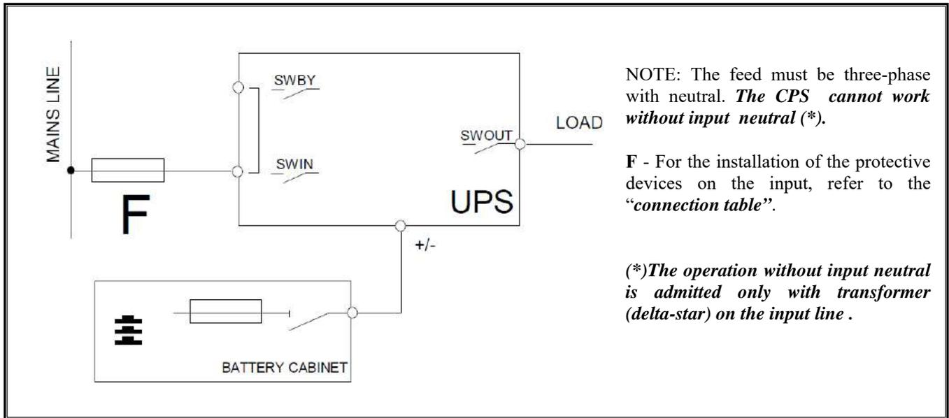
The links between the SWIN and SWBY switches are pre-fitted.
