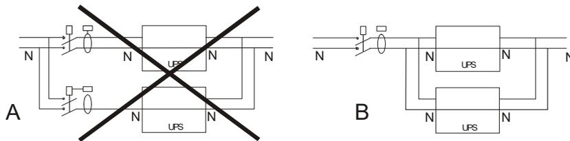
In order to avoid unnecessary interventions, versions with several parallel-connected devices must have a single differential switch inserted at the input of the whole system, as shown in figure B.
