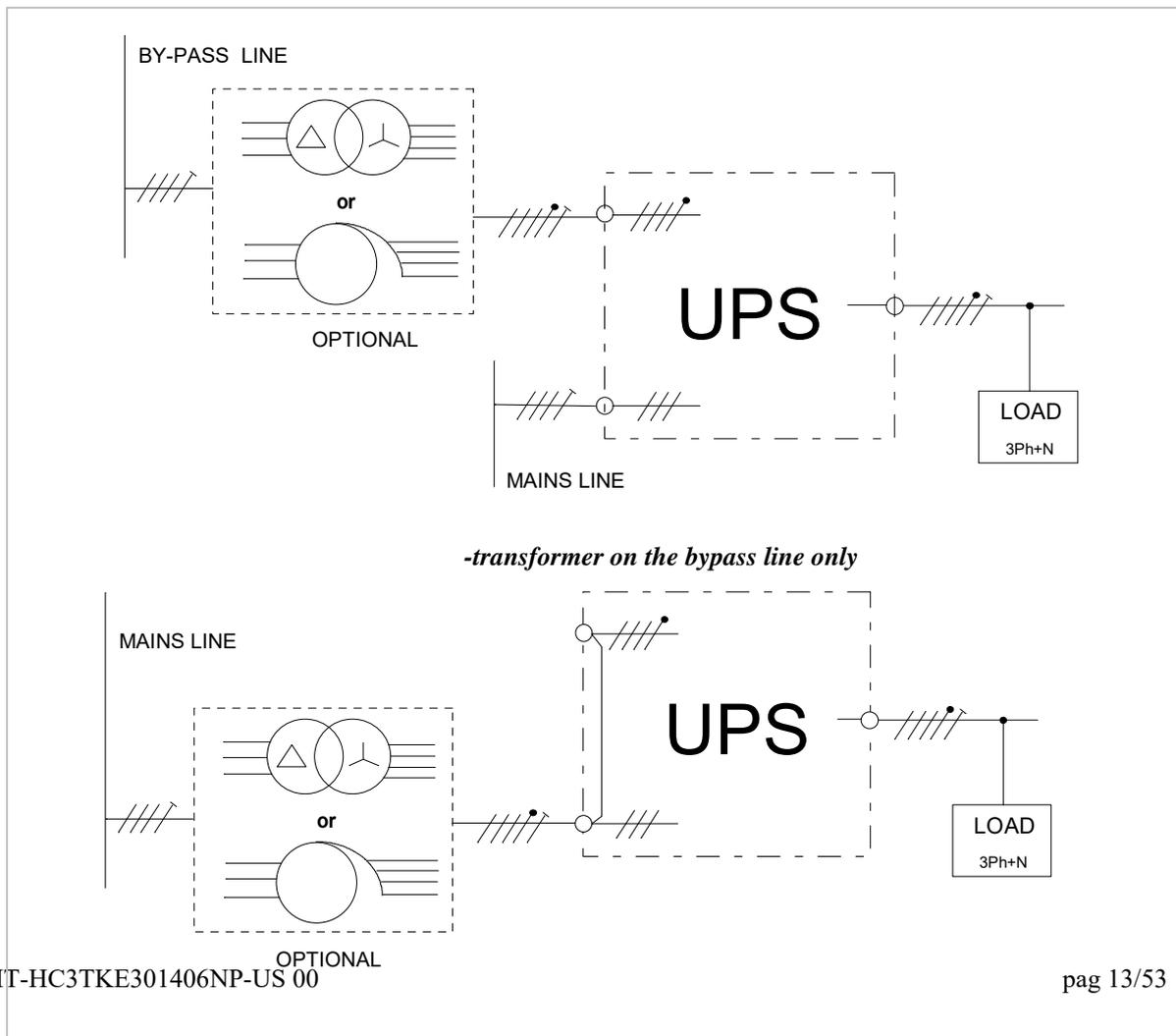
*-The transformer supply bypass and mains lines*
