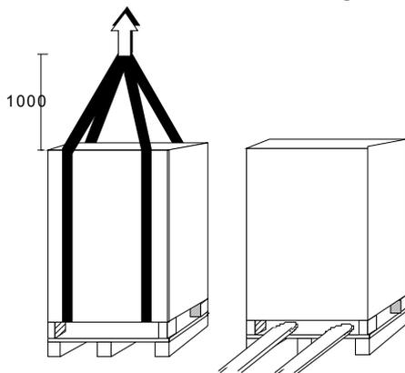
RIMOZIONE DEL PALLET / TO REMOVE THE PALLET
