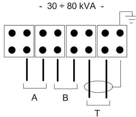
The contacts of each disconnector must be connected to the corresponding CPS terminals, as shown in the diagram.
