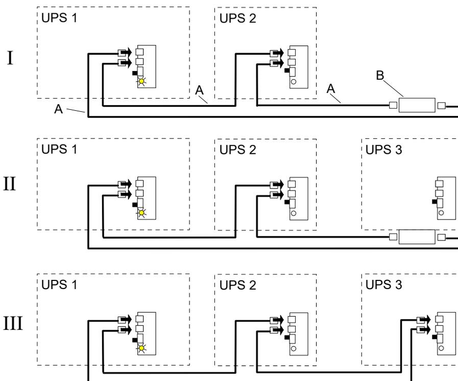
A) CPS parallel cable type RJ45
