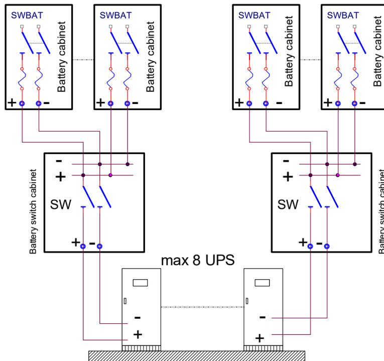
**TO CONNECT MORE CPS IN PARALLEL WITH ONLY ONE BATTERY:**
