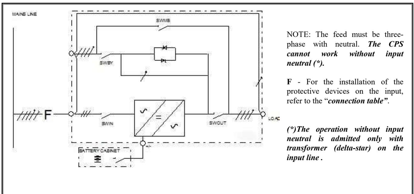
The links between the SWIN and SWBY switches are pre-fitted.
